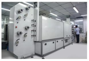
Continuous Annealing Furnace 连续退火炉
